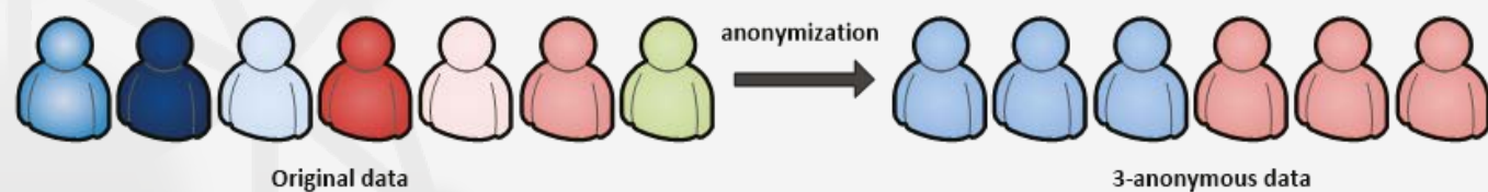
Figure 2. A piece of data has k -anonymity properties if the information for each subject in the dataset cannot be distinguished from at least k-1 individuals, being k a parameter of choice.
